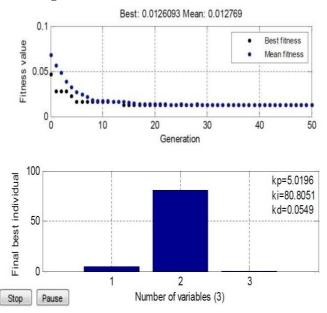
Figure 10: GA optimization progression based objective function (IAE) index
