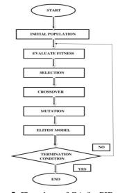
Figure 5: Flowchart of GA for PID tuning
