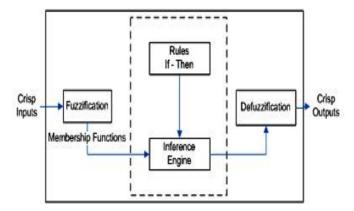
Figure 6: Configuration of Fuzzy Logic Controller
