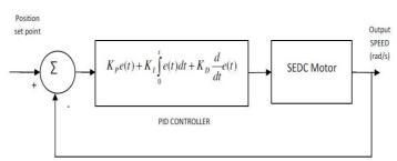
Figure 3:PID Controller with System
